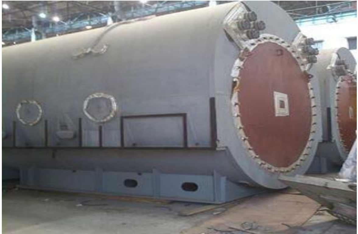
Fig 8: Stator Core Frame
