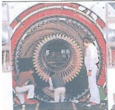
Laying Of Water Cooled Winding In the Stator Of 500 MW Turbo Generator
